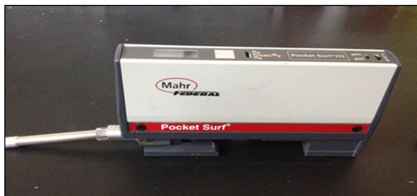
Figure 4: Profile-meter for measuring (SR)
