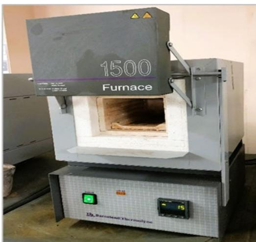
**Figure 1:** Barnstead Small Electric Benchtop Muffle Furnace
