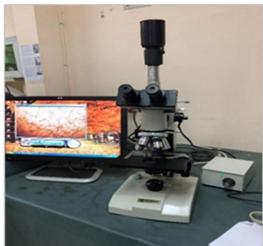
**Figure 2:** EUROMEXPB-4161 Metallurgical Microscope
