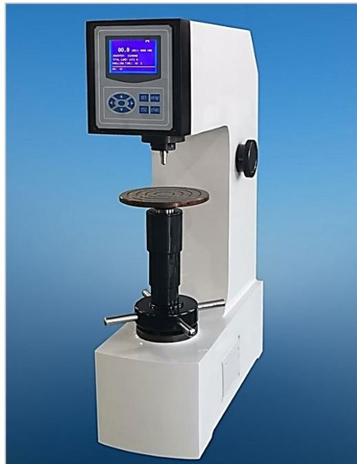
Figure 4: Rockwell Hardness Tester machine, HRS-150 digital
