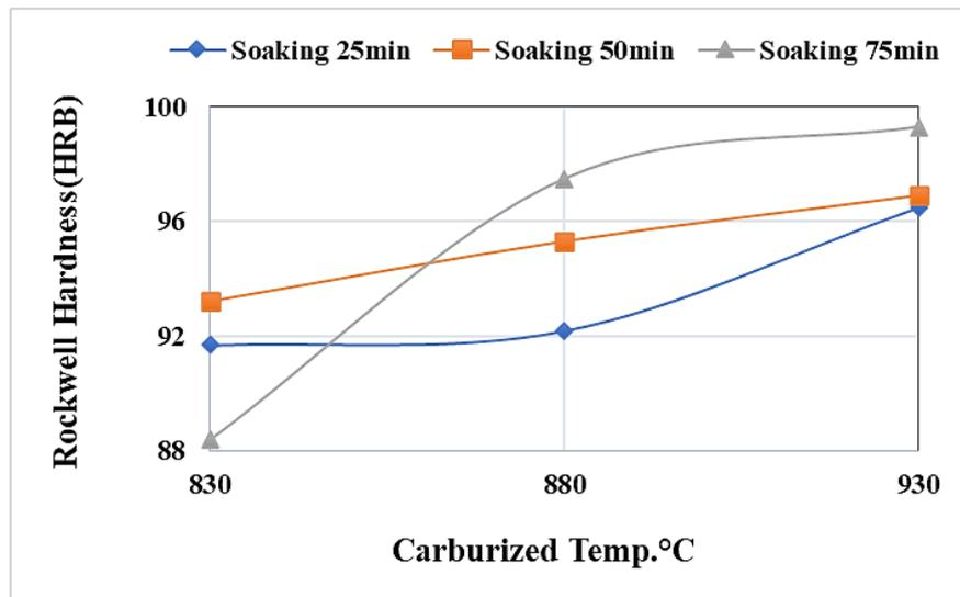
Figure 8: The influence of carburized temperature and soaking duration on hardness
