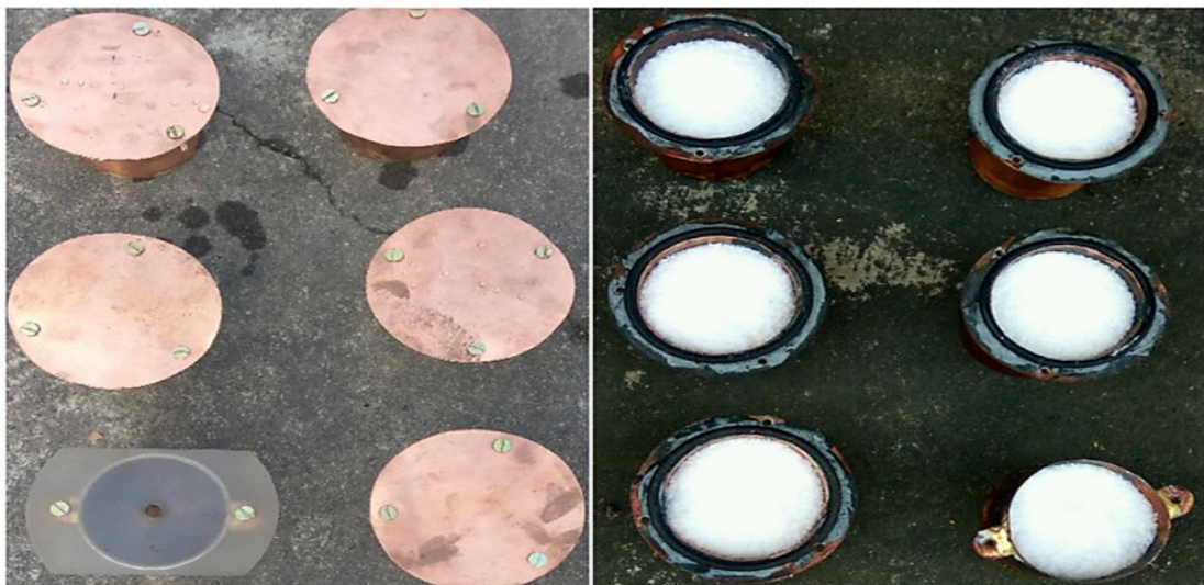
Figure 8: Pictorial view of PCM-loaded copper cylinders [83]
