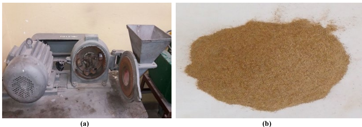
Plate 3: (a) Table top harmer mill for crushing of raffia palm fibres (b) Crushed powdered sample of raffia palm fibre
