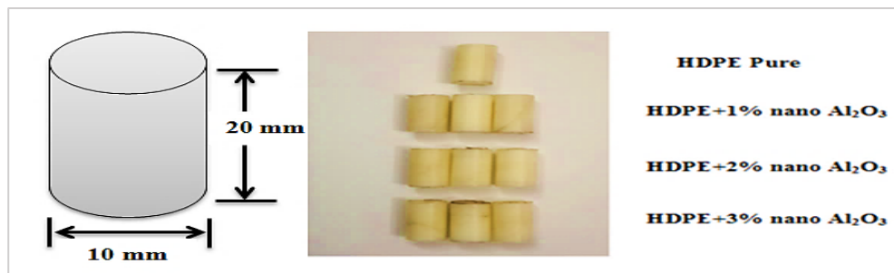
Figure 2: Standard and actual wear test specimens
