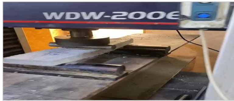
Figure 7: (PVA-ECC) concrete plate tested at (28) days
