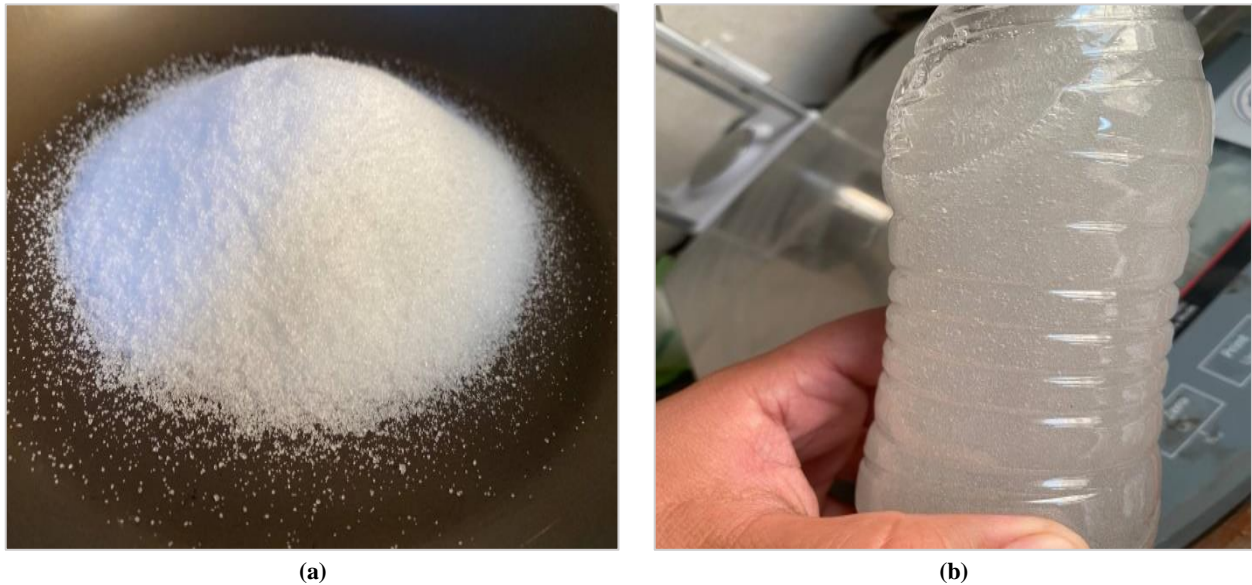
Figure 4: Polyvinyl Alcohol solution (PVA) solution preparation.
