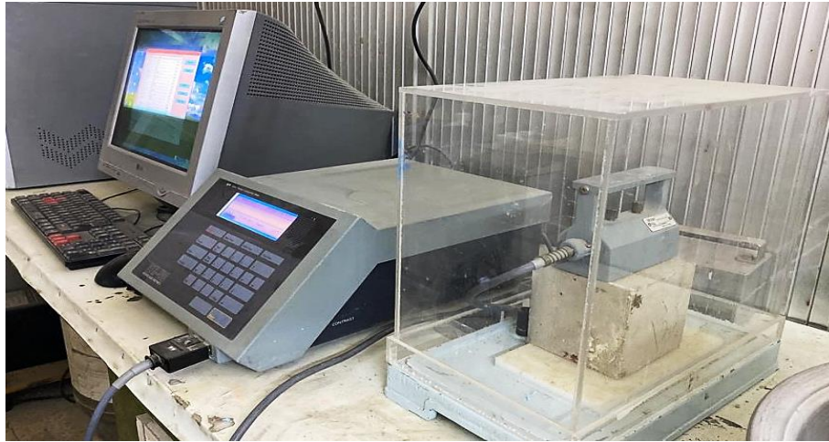
Figure 9: Thermal conductivity test by using cube (100×100×100) mm
