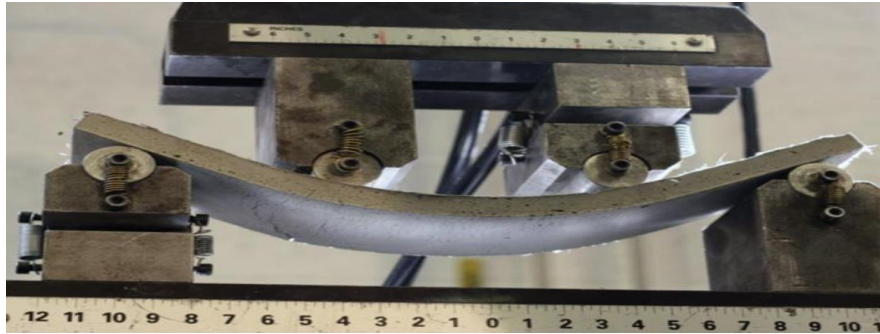
Figure 2: Response of ECC under flexural loading [30]
