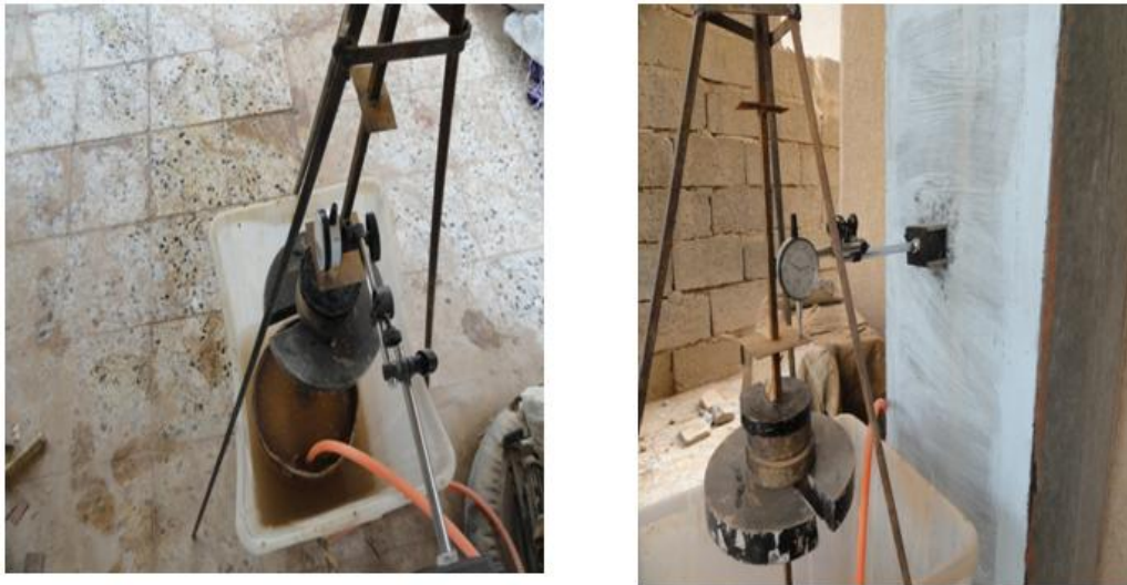
Figure (2): Laboratory model preparation and equipments for soaking and leaching Sabkha soil.
