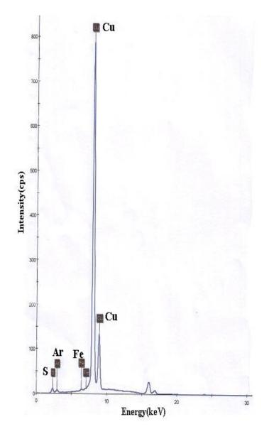
Figure (4) XRF of copper carbonate CuCO<sub>3</sub>·Cu(OH)<sub>2</sub> powder prepared by method of microemulsion process. The high purity concentration of the copper while other peaks of material could be neglected for their count rates.
