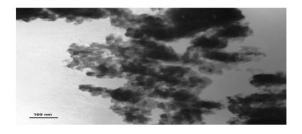
(a) Figure (1) a - TEM image for CuCO<sub>3</sub>·Cu(OH)<sub>2</sub> nanoparticles synthesized by method microemulsion process the particle size about (10-50 nm).
