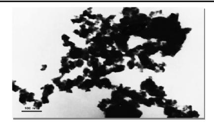
(b) Figure (1) b -TEM image for copper CuO nanoparticle synthesized by method microemulsion process, the particle size about (10-50 nm).
