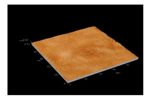
Figure (2) AFM high magnification micrograph, super transparent, CuO thin-film coated deposited on glass substrate by using of ultrasonic spray pyrolysis technique, the Root mean square (0.228 nm).
