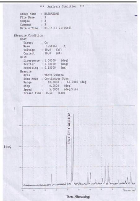
Figure (3) XRD patterns of copper carbonate  $CuCO_3 \cdot Cu(OH)_2$  powder prepared by method of microemulsion process,  $2\Theta(29)$  [6]. The particle size of powder by use (Debye-Scherr's) equation that the particle size of powder a range about (30-40) nanometer[7].
