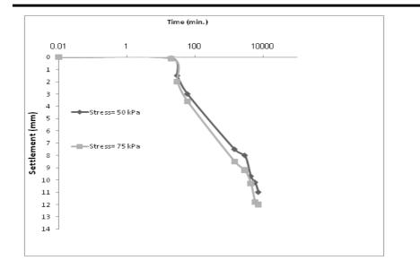
Figure (4): Time- settlement curves for sabkha soil without treatment.
