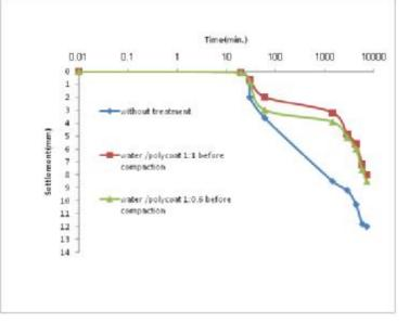
Figure (7): Time-settlement curves for sabkha soil without Treatment and with addition of polycoat (Stress=75kPa.).
