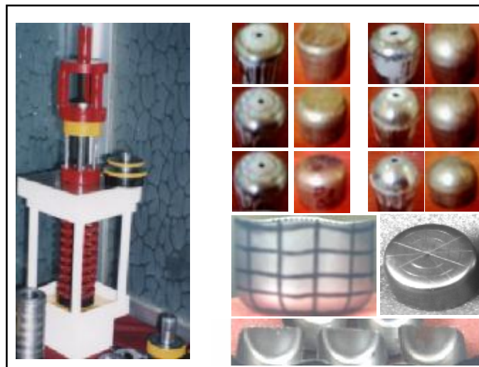
FIG ( 2 ) : Drawing die used in the experimental work, completely drawn parts (produced cup) , divided part & the distortion of grid circles at the cup wall & bottom.
