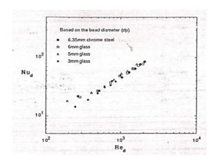
Fig(9) Average Nusselt Number (Nu<sub>d</sub>) in apacked channel<sup>[5]</sup>
