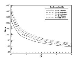
Fig (4) Local Nusselt number variation with the horizontal coordinate for Carbon dioxide
