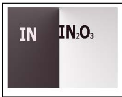
Fig. (3): A photograph of an \text{In}_2\text{O}_3 film prepared by thermal oxidation
