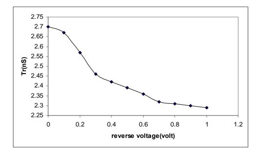
Fig.(8) Raise time detector as function of bias voltage
