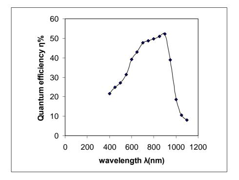
Fig.( 3 )Relative Quantum Efficiency of PIN as function of Wavelength
