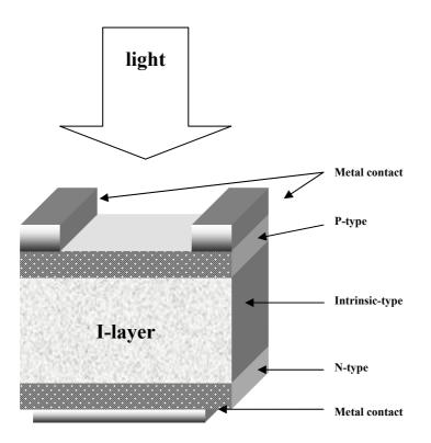
Fig. (1) show diagram of PIN photodetector
