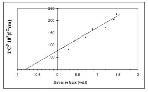
Fig.(7) C<sup>-3</sup> as function a of reverse bias voltage.
