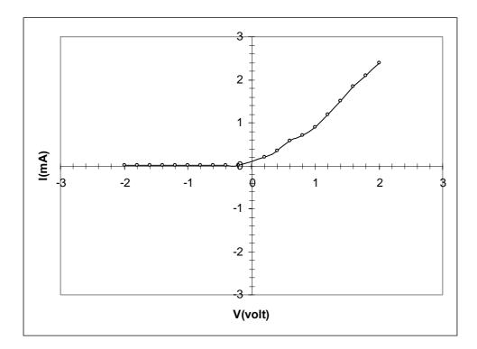
Fig.( 4) I-V Characteristics of PIN Photodetecter
