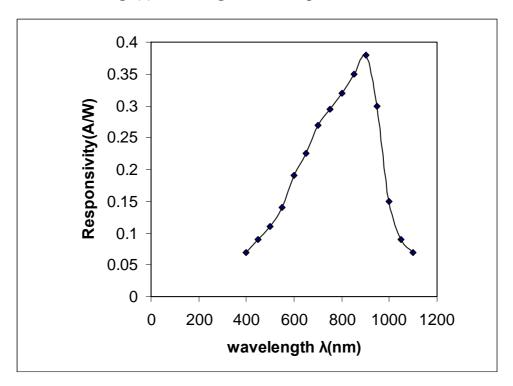
Fig.(2) Spectral Response of PIN Photodetector
