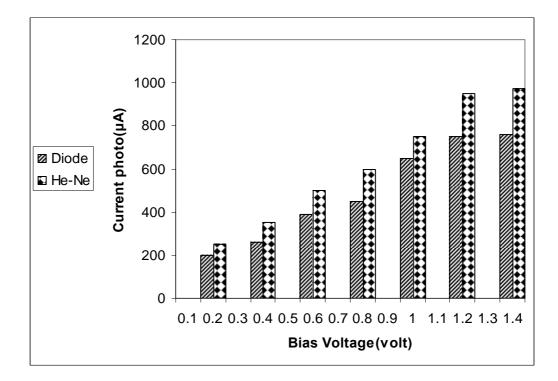
Fig. (5)Spectral Response of detector for two laser He-Ne and diode have power 1mW as function of bias voltage
