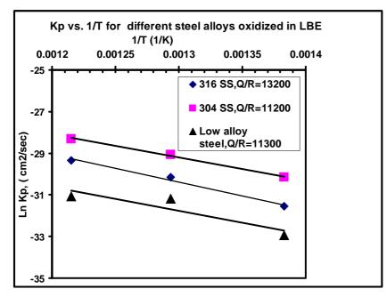
Figure( 5). The parabolic rate constant (*Kp*) vs. (1/T) for different steels oxidized in LBE at 450-550 °C for 100 hrs..
