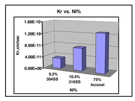
Figure( 6) Scale removal rate constant vs. Ni% for different alloys oxidized at
