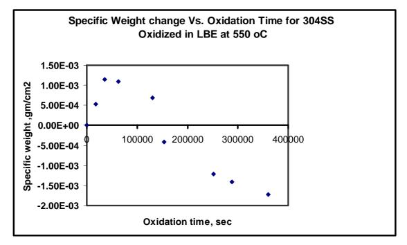
Figure (3). Specific weight change versus oxidation time for 304 SS at 550  $^{\circ}\mathrm{C}$
