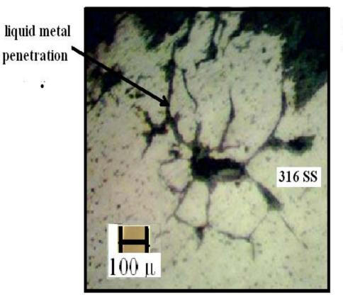
Figure (8) . Lead-Bismuth penetration in 316SS after 100 hrs oxidation at 550 °C.
