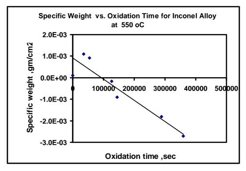
Figure (2). Specific weight change versus oxidation time for inconel 600 at
