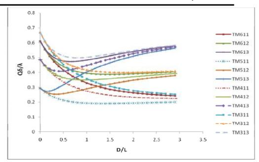
Figure (3)  $(Q\delta/\lambda)$  versus (D/L) for several modes in a right circular cylindrical cavity.
