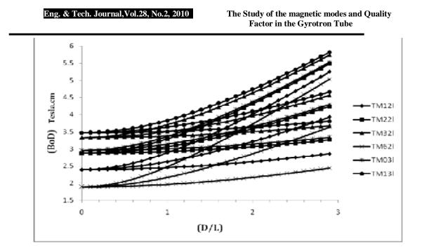
Figure (4b) shows a relation between the applied magnetic field and the cavity dimension for each  $TM_{mnl}\mathchar`$  mode.
