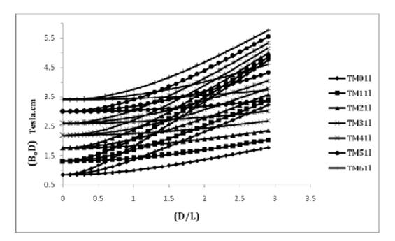
Figure (4a) shows a relation between the applied magnetic field and the cavity dimension for each  $TM_{mnl}$ - mode.
