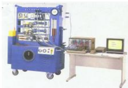
Figure (2) Photograph of electro-hydraulic control unit test bench
