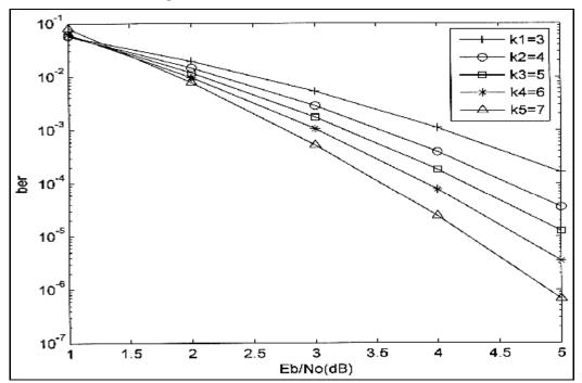
Figure (7) simulated performance results for 1/2 rate RSC code in soft decision viterbi decoding for different constraint length
