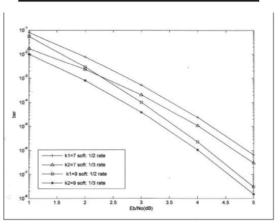
Figure (10) simulated performance results for 1/2 and 1/3 rates RSC code in soft decision viterbi decoding for constraint length (7, 9)
