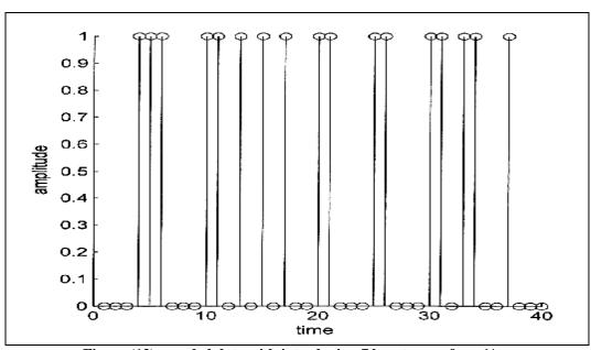
Figure (13) encoded data with introducing 7 burst error from ½ rate RSC encoder without interleaver
