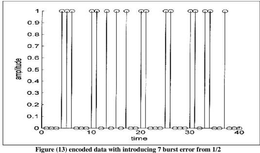
rate RSC encoder with interleaver
