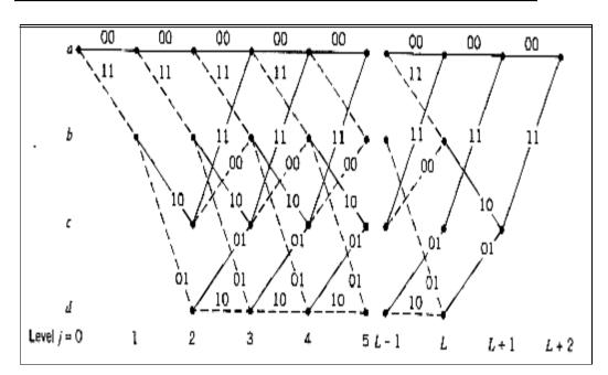
Figure (2) trellis for the convolutional encoder of figure 3
