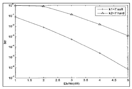
Figure (9) simulated performance results for 1/2 rate, 7 constraint length RSC code in soft and hard decision viterbi decoding
