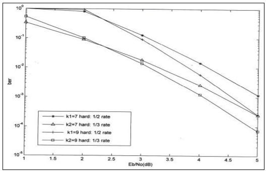
Figure (11) simulated performance results for 1/2 and 1/3 rates RSC code in hard decision viterbi decoding for constraint length (7, 9)
