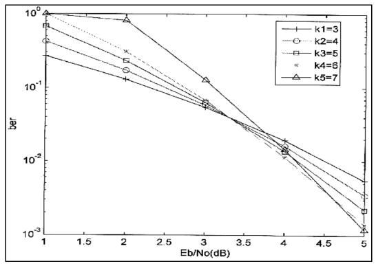
Figure (8) simulated performance results for 1/2 rate RSC code in hard decision viterbi decoding for different constraint length
