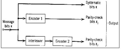
Figure (4) block diagram of turbo code
