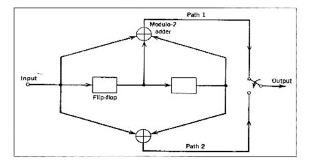
Figure (3) constraint length-3, rate-1/2 convolutional encoder
