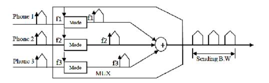
Figure (4) FDM Multiplexing Process in Frequency Domain.
