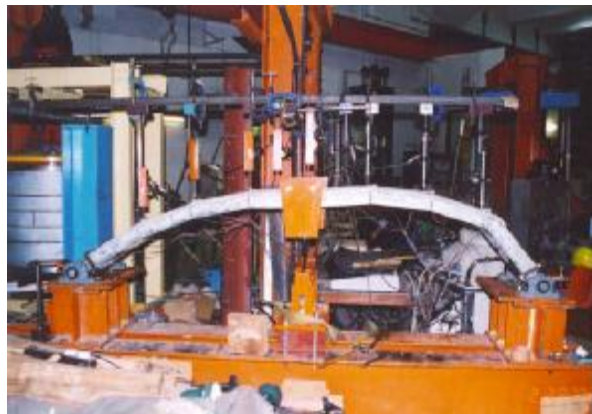
Figure (3) Failure mode of a composite arch [4]
