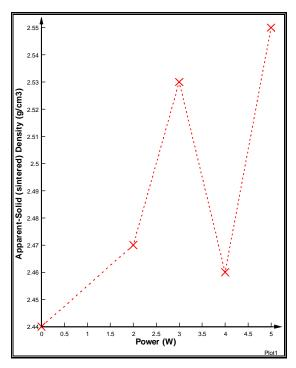
Figure (7) Power and apparent-solid (sintered) density
