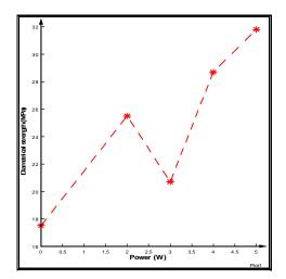
Figure (4) Shows the relation between Power and Diametrical strength
