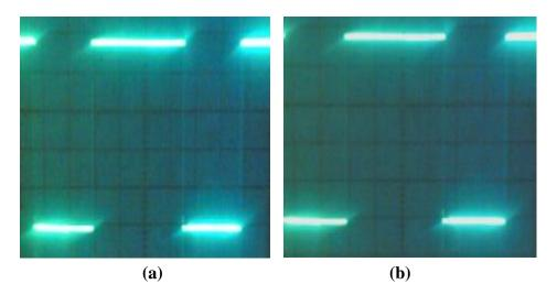
Figure (4) Illustrates the (a) unlaunched signal 7.2ms (138.889Hz) and (b) launched signal 7.22ms (138.405Hz) (1V/div, 2ms/div).
