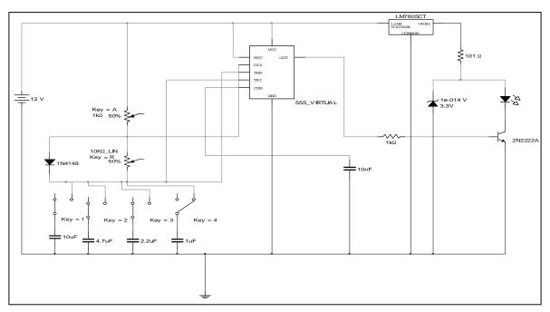
Figure (2) Transmitter circuit diagram
