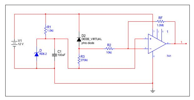
Figure (3) Optical fiber receiver
