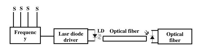
Figure (1) Block diagram of optical fiber arrangement.
