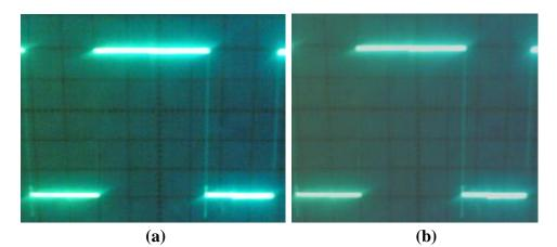
Figure (6) shows the unlaunched and transmitted signals (a) the unlaunched signal is of (645.1613Hz) 1.55ms pulse width. (b) the transmitted signal is of (643.0868Hz) 1.555ms pulse width (1V/div, 0.5ms/div). 1414
