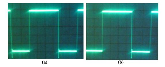
Figure (7) Pulse shapes of (a) the unlaunched signal of a pulse width (0.73ms), and frequency (1369.86Hz) and (b) of the transmitted signal of pulse width (0.732ms), frequency (1366.120Hz) (1V/div, 0.2ms/div)
