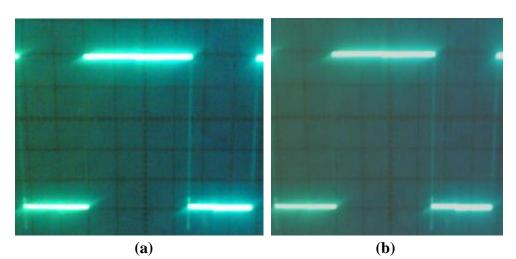
Figure (5) Demonstrates the (a) input signal before being launched (277.778Hz, 3.6ms) (b) the output signal after being transmitter into the fiber (277.008Hz ,3.61) (1V/div, 1ms/div).
