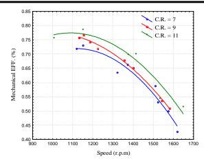
Figure (7) Effect Variable Compression ratio on Mechanical Efficiency as a Function of Engine Speed.
