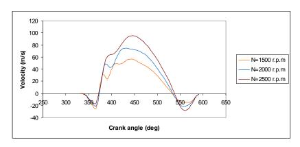
Figure (15) Velocity variations in the air pipe during gas exchange period at pipe end no.3.
