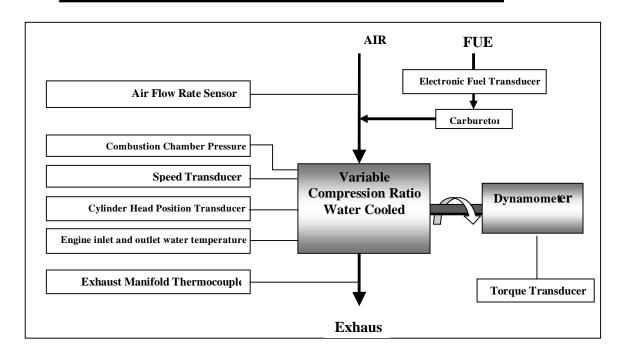
Figure (2)-B Schematic diagram for the variable compression engine
