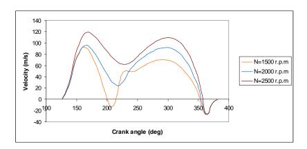
Figure (16) Velocity variations in the exhaust pipe during gas exchange period at pipe end no.1.
