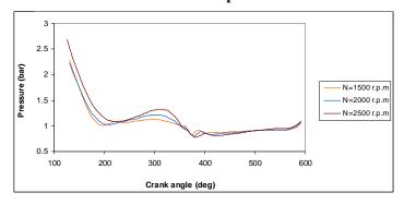
Figure (9) Pressure variations inside the cylinder during gas exchange period at different speeds with CR =9.
