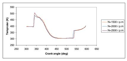
Figure (13) Temperature variations in the air pipe during gas exchange period at pipe end no. 3.
