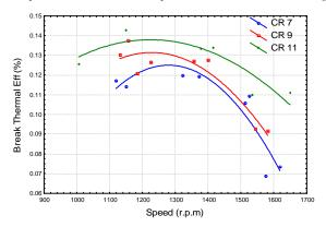
Figure (5)Effect Variable Compression ratio on Brake Thermal Efficiency as a Function of Engine
