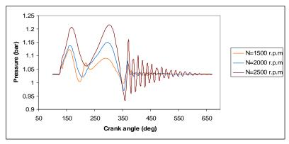
Figure (12) Pressure variations in the exhaust pipe during gas exchange period at pipe end no. 1.
