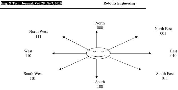
Figure (6) Direction of robot movement
