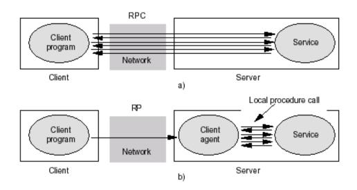
Figure (2) <u>a</u> Remote procedure call and <u>b</u>Remote programming
