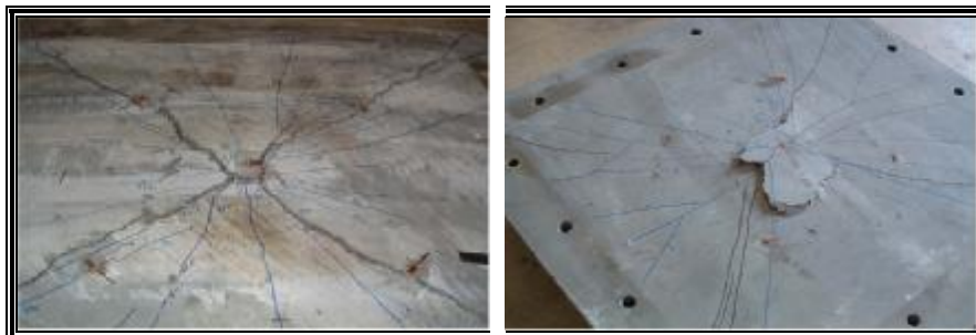
a. Failing in Flexure
