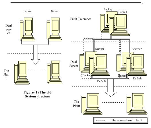
Figure (2) proposed System structure
