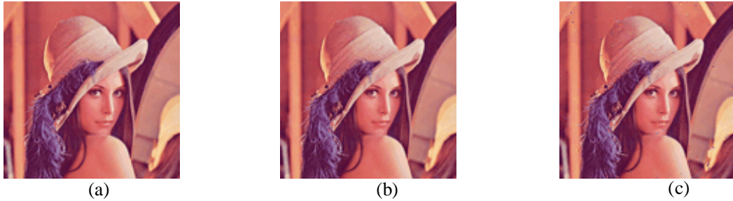
Figure (11): lenna image with a block size 2x2 (a) cover-image, (b) stego-image without substitution, (c) stego-image with substitution
