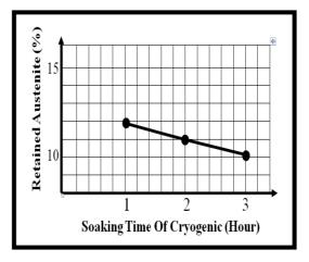
d) show the relation between soaking time of cryogenic & retained austenite for specimens (C8, C9 & C10).
