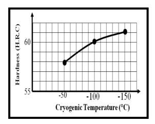
a).<br/>show the relation between cryogenic temperature & hardness for specimens<br/>  $(C1,\,C2$  & C3)
