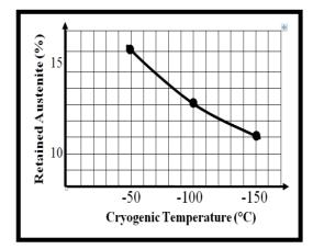
a) show the relation between cryogenic temperature & retained austenite for specimens (C1, C2 & C3)
