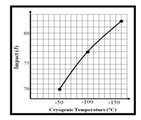
c) show the relation between cryogenic temperature & impact for specimens (C6, C7 & C8).
