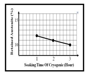
b) show the relation between soaking time of cryogenic & retained austenite for specimens (C3, C4 & C5)
