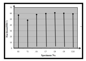
Figure (2) shows the plot of hardness as function of the different thermal process sequence in oil hardening.
