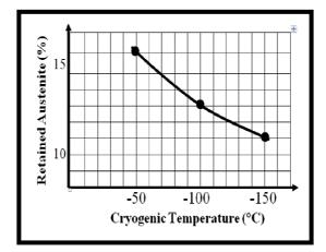
c) show the relation between cryogenic temperature & retained austenite for specimens (C6, C7 & C8).
