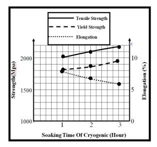
b) show the relation between soaking time of cryogenic & tensile strength for specimens (C3, C4 & C5)
