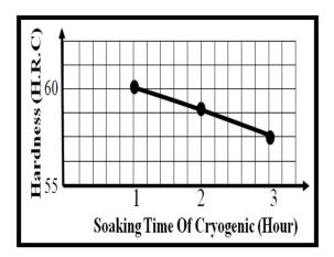
b) show the relation between soaking time of cryogenic & hardness for specimens (C3, C4 & C5)
