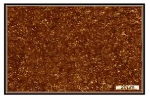
f. show the microstructure for specimen (C5) with retained austenite  $(10\%)\,\text{-}1000\text{X}$
