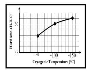
c) show the relation between cryogenic temperature & hardness for specimens (C6, C7 & C8).
