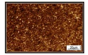
m) show the microstructure for specimen (C10) with retained austenite (8%) -1000X
