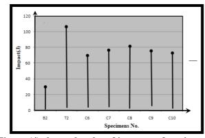
Figure (4) shows the plot of impact as function of the different thermal process sequence in oil hardening
