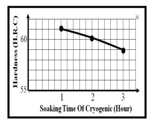
d) show the relation between soaking time of cryogenic & hardness for specimens (C8, C9 & C10).
