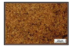
k) show the microstructure for specimen (C8) with retained austenite (11%) -1000X
