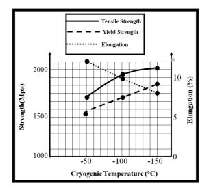
a) show the relation between cryogenic temperature & tensile strength for specimens (C1, C2 & C3)
