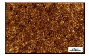
l) show the microstructure for specimen (C9) with retained austenite (10%) - 1000X
