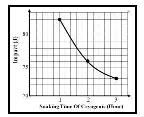
d) show the relation between soaking time of cryogenic & impact for specimens (C8, C9 & C10).
