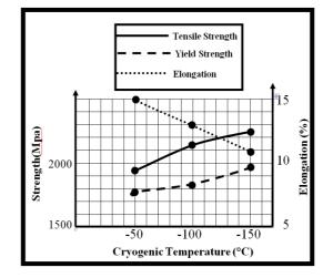
c) show the relation between cryogenic temperature & tensile strength for specimens (C6, C7 & C8).
