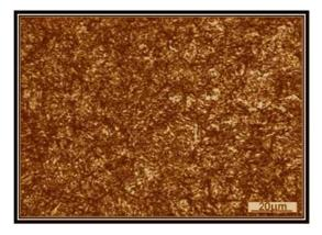
c) show the microstructure for specimens (C3) with retained austenite (12%)  $-1000 \mathrm{X}$
