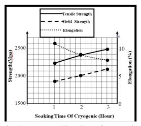
d) show the relation between soaking time of cryogenic & tensile strength for specimens (C8, C9 & C10).
