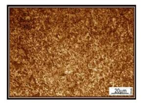
g) show the microstructure for specimen (C6) with retained austenite (16%) -1000X
