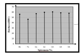
Figure (1) shows the plot of hardness as function of the different thermal process sequence in air hardening.
