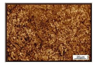
h) show the microstructure for specimens (C7) with retained austenite (13%) -1000X
