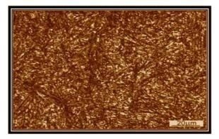
b) show the microstructure for specimen (C2) with retained austenite (15%) -1000X
