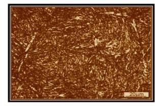
a) show the microstructure for specimen (C1) with retained austenite (18%)  $-1000\mathrm{X}$
