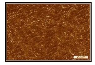
d) show the microstructure for specimen (C4) with retained austenite (11%) -1000X
