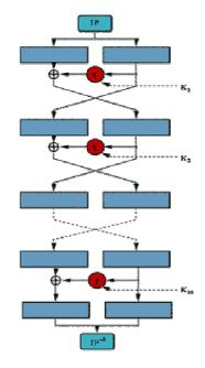
Figure (1) General design of a Feistel cipher
