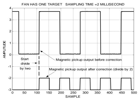
Figure (9) Magnetic pickup signal after correction.
