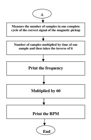
Figure (11) Flowchart for measuring frequency & RPM.
