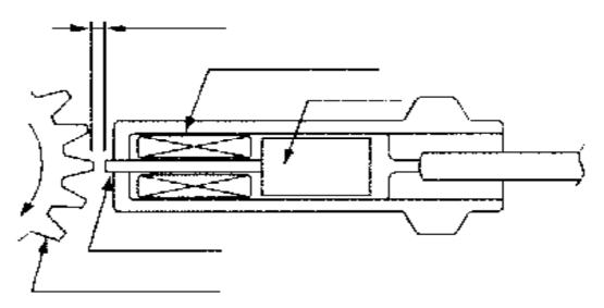
Figure (1-a) External construction of the magnetic pickup [2].
