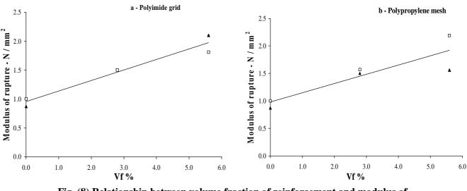
Fig. (8) Relationship between volume fraction of reinforcement and modulus of rupture for concrete sandwich panels
