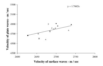
Fig. (2) Relationship between plate and surface wave velocities for concrete sandwich panels
