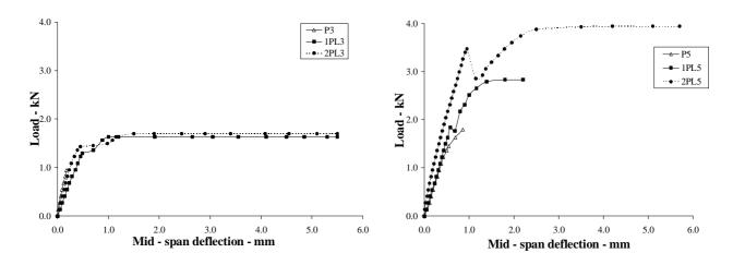
Fig. (5) Load – deflection curves at mid – span for concrete sandwich panels in series (4) and (5)
