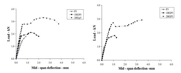
Fig. (6) Load – deflection curves at mid – span for concrete sandwich panels in series (6) and (7)
