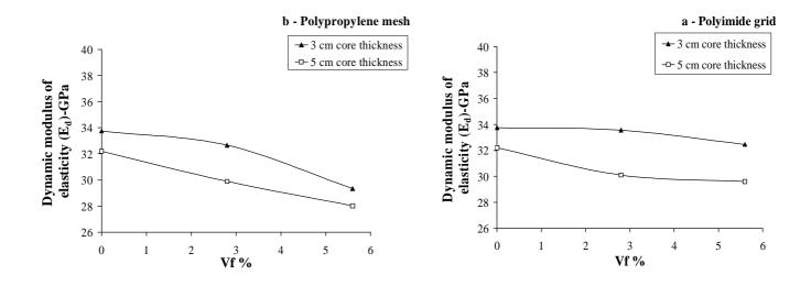
Fig. (3) Relationship between volume fraction of reinforcement and dynamic modulus of concrete sandwich panels
