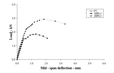
Fig. (7) Load – deflection curves at mid – span for concrete sandwich panels in series (8)
