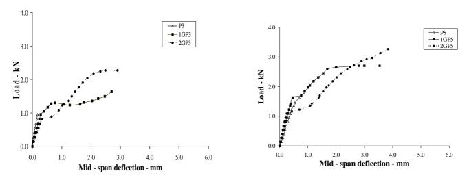
Fig. (4) Load – deflection curves at mid – span for concrete sandwich panels in series (2) and (3)
