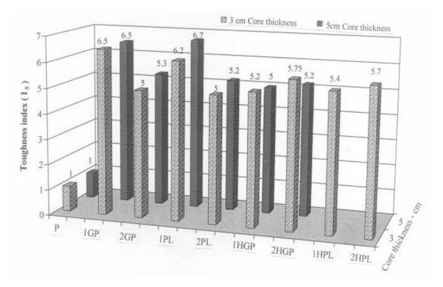
Fig. (9) Comparison of toughness index (I<sub>5</sub>) of concrete sandwich panels
