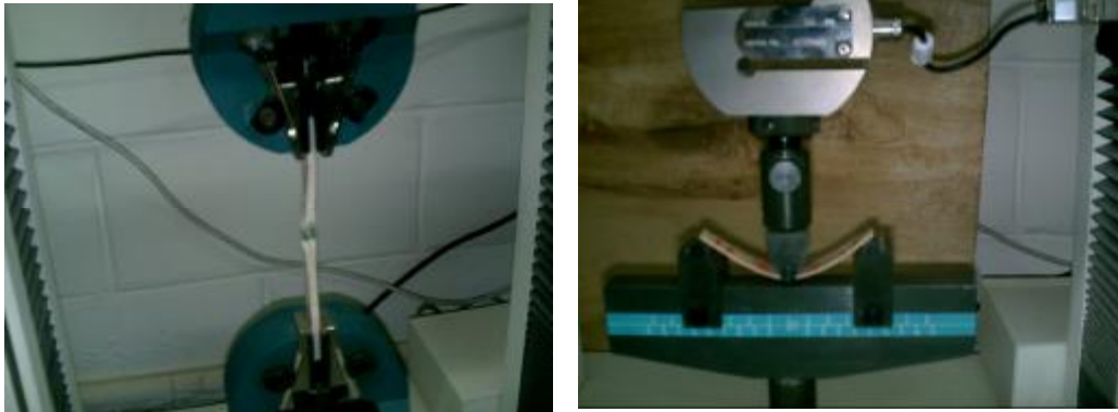
a) Specimen under tensile test
