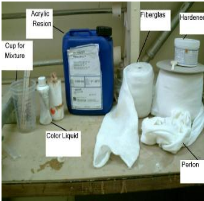
a) Materials used for above knee socket lamination b) Positive mold with vacuum system
