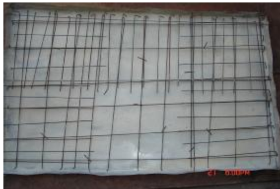
Photo (7) Details of the reinforcement mesh of slab S_8 (case8).
