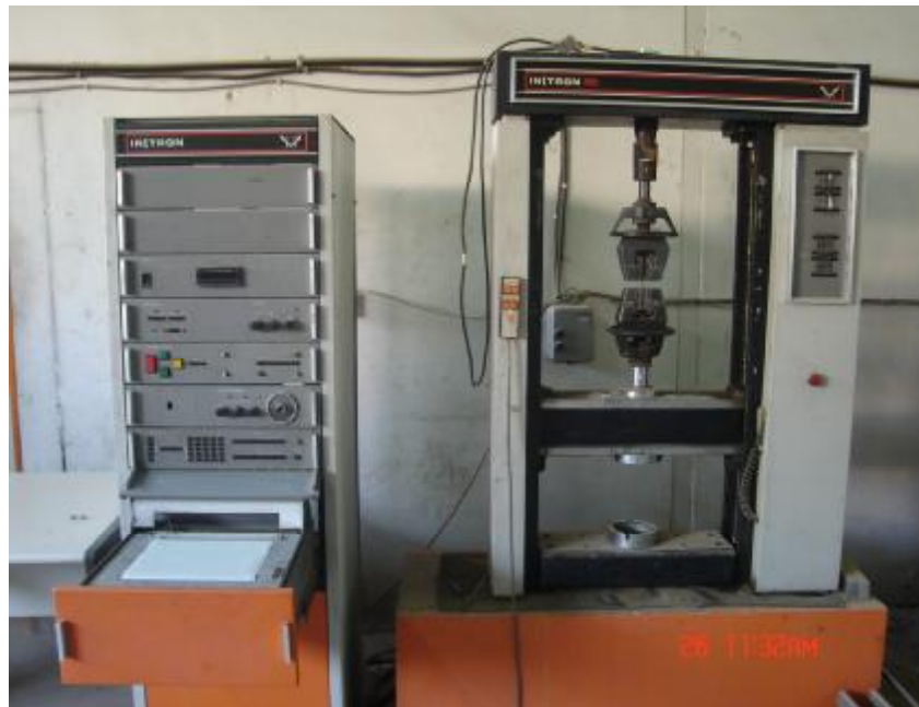
Photo (1) The tensile testing machine belonging to the laboratory of the Department of Minerals and Production Engineering in the University of Technology which has been used in the present study.
