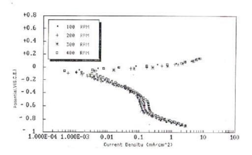
Figure(4): Potentiostatic polar curves of deareated solution,temp.293K
