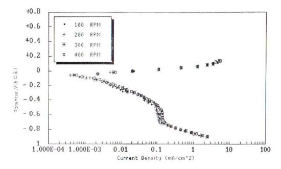
Figure(3): Potentiostatic polar curves of deareated solution, temp.288K
