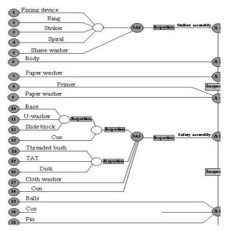
Figure (4) Assembly Chart For the
