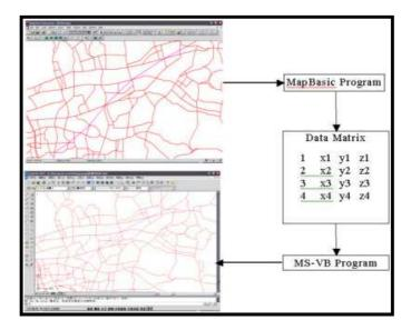
Figure (7) Structure of Data Transfer from MapInfo to AutoCAD [3]
