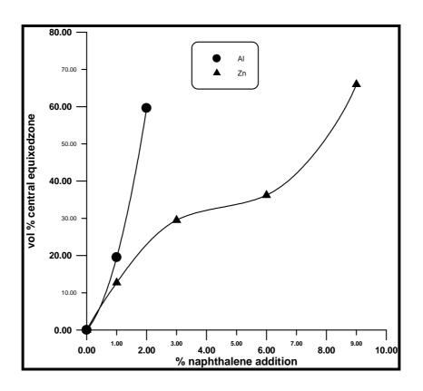
Figure (3) Effect of naphthalene addition on the % volume of equiaxed grains in the structure
