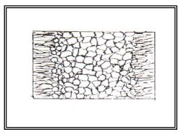
(e) 9% naphthalene Figure (2) Ingot structure of commercially pure Zinc with different naphthalene additions.
