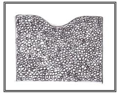
Figure (4) Ingot structure of commercially pure aluminum cast from (40°C) super heat.
