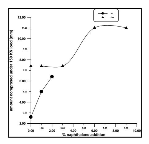
Figure (5) Compressed height under 150 KN loads as a function of naphthalene addition.
