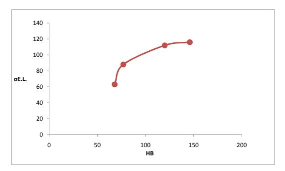
Figure (5) Fatigue strength against HB at different temperatures (room temperature to 300°C)
