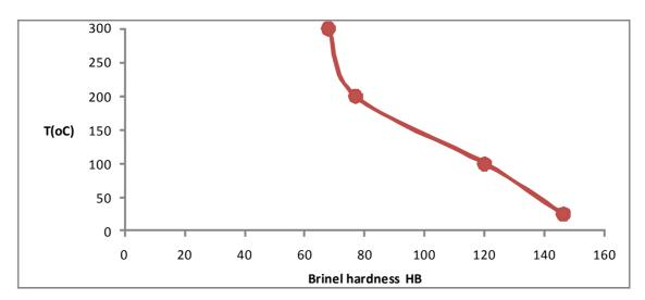
Figure (4-B) shows the variation of temperature with the HB hardness of copper alloy
