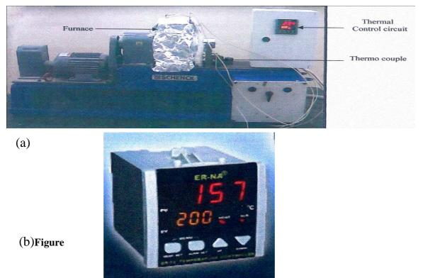
(3): (a) furnace attached with fatigue machine (b) ER-NA temperature controller [8]
