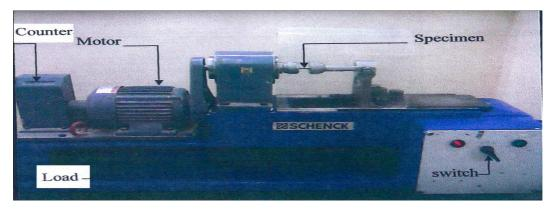
Figure (2): PUNN Rotary Fatigue bending machine [8]
