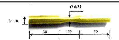
Figure (1) : shows the geometry of fatigue creep interaction specimens, dimensions in (mm)
