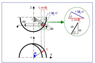
Figure (4) Un-cut chip thickness
