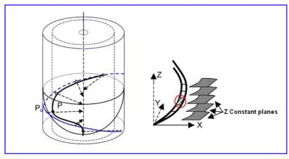
Figure (1) Cutting edge discretization [12]
