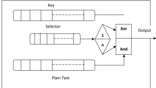
Figure (5) Operation By elements selector
