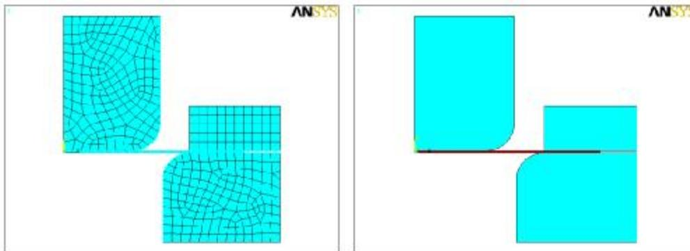
Figure (2) FE Model of axisymmetric deep drawing
