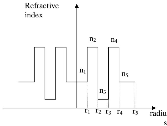
Figure (1): Index profiles Five-layer fiber structure
