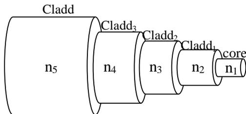
Figure (2): five layer cylindrical dielectric structure
