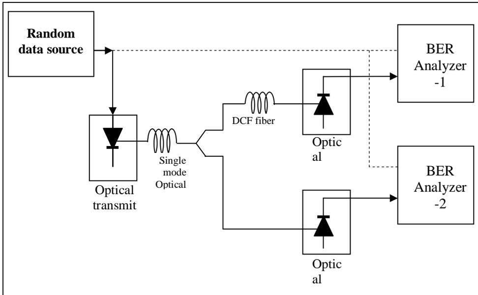
Figure(5): The experiment setup of optical fiber communication system with using DCF.
