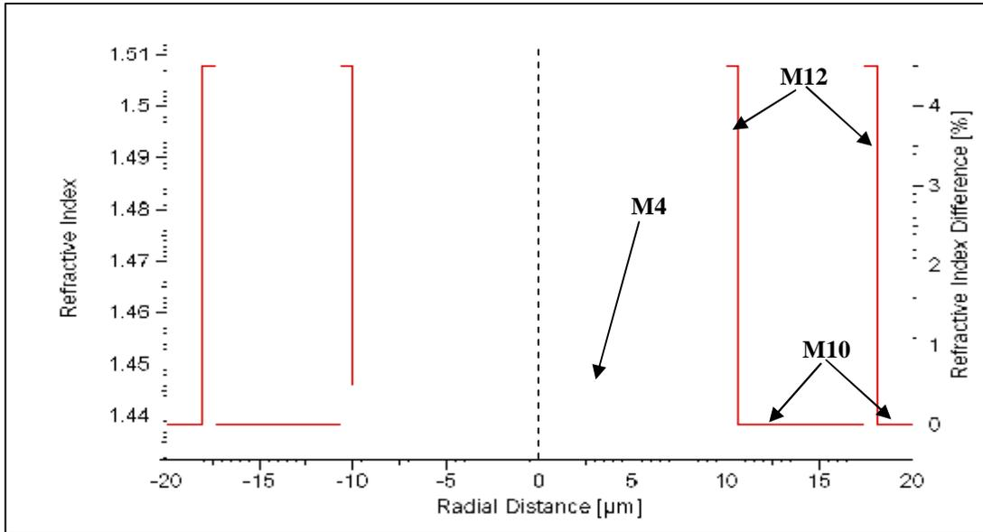
Figure(3): Index profiles of proposed five layers fiber structure
