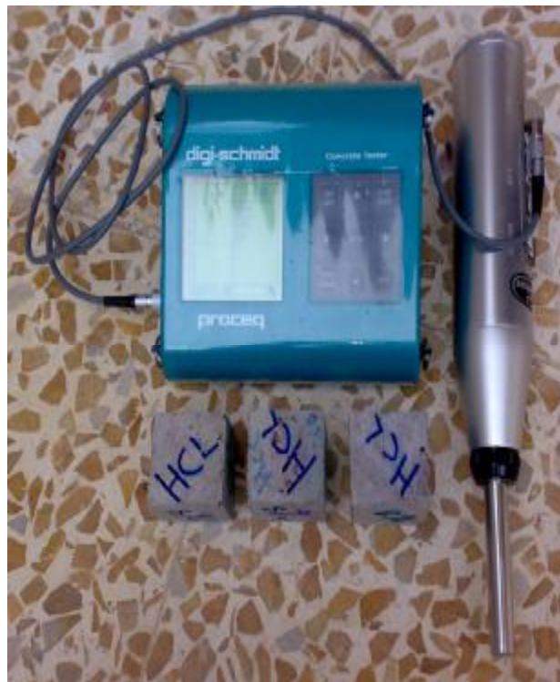
Figure (7) Hammer test of rubberize cement mortar cubes
