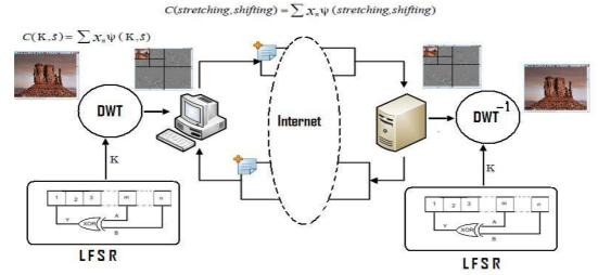
Figure 5: Randomized Dyadic Dilation DWT based Authentication Scheme
