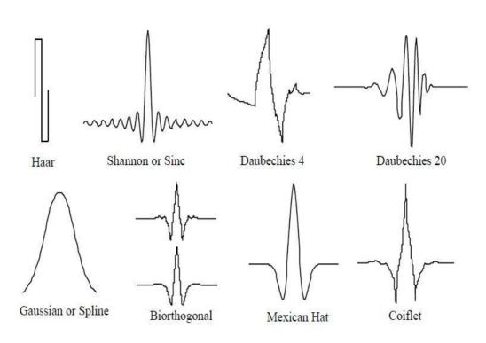
Figure 4: Different Types of Wavelet Signals
