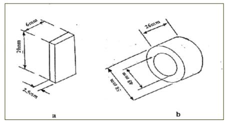
Figure (1): a. Test Pin b. Test Journal.
