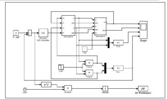
Figure (5) PID Controller of the S.G.
