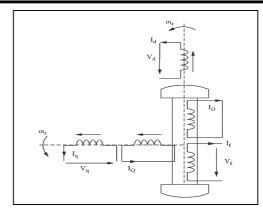
Figure (1) S.G. Windings in dq-axis
