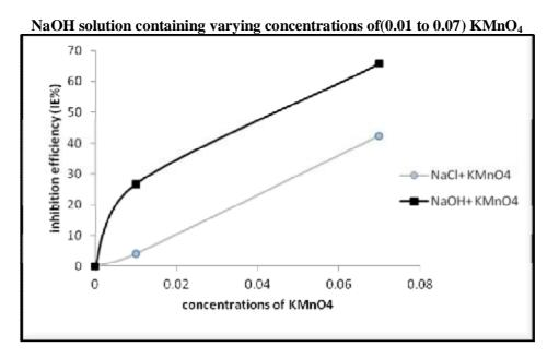
Figure 3. inhibition efficiency (IE%) with concentration of KmnO<sub>4</sub>
