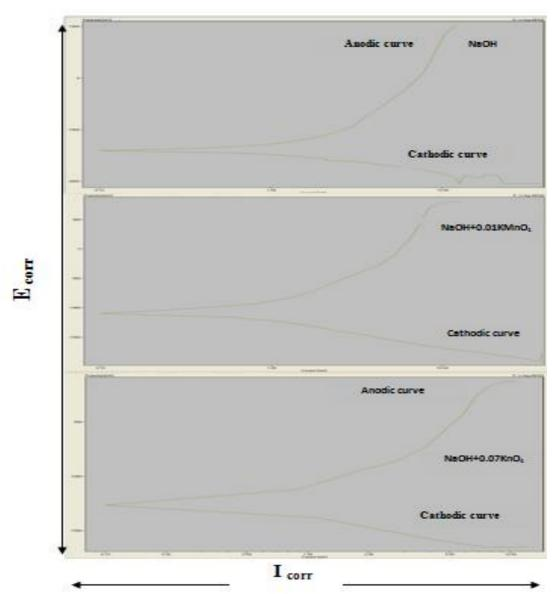
Figure (1) Potentiodynamic polarization curve of brassin (0.6M) NaCl solution containing varying concentrations of (0.01 to 0.07) KMnO<sub>4</sub>
