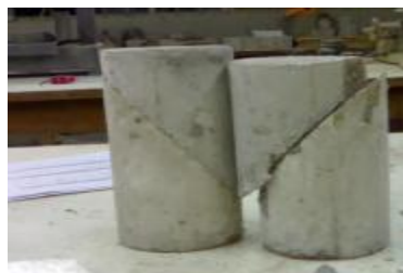
Figure (6) Slant Shear Failure Mode of M_{S,B,R} with C_{25} Composite Cylinder Specimens at 28 Days Age.
