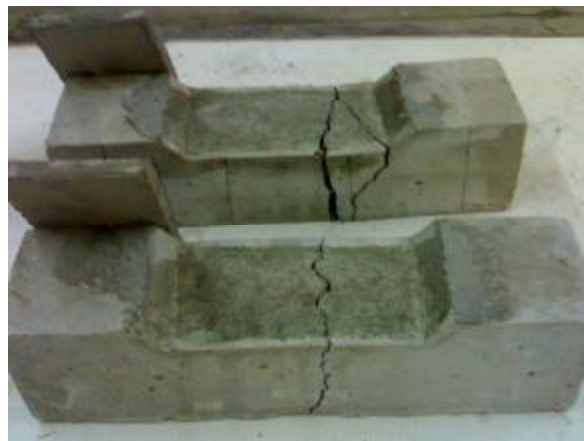
Figure (9) Prism Composed of C_{25} Repaired by M_{S.B.R} , 28 Days Age.
