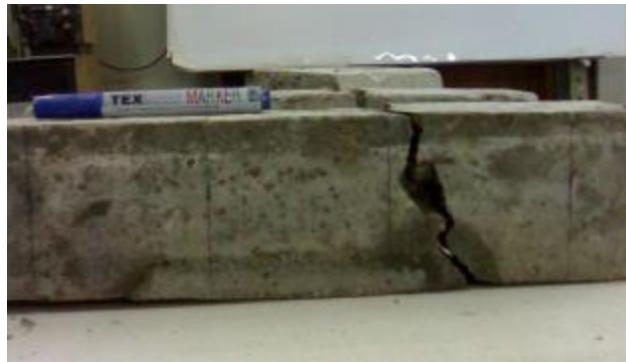
Figure (8) Prism Composed of C_{15} Repaired by M_C , 28 Days Age.
