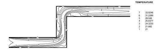
(b) H/W=3, U<sub>in</sub>=0.14 m/s, T<sub>w</sub>=35°C
