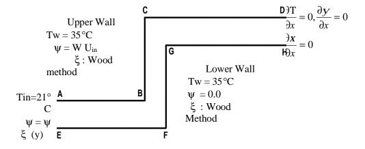
Figure (2) Boundary conditions for laminar flow at H/W=3.
