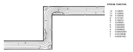
(c) H/W=4, U<sub>in</sub>=0. 5m/s, To=40°C
