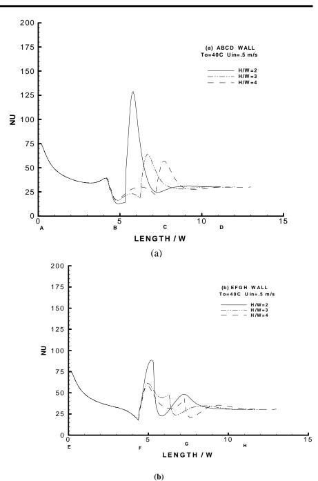
Figure 11 Local Nusselt number distribution along the upper and lower duct walls, U<sub>in</sub>=0.5 m/s, To=40 °C, and (H/W=2, 3, and 4).
