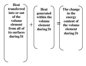
repeating for each  $\Delta t$  until the solution at the desired time is obtained [14, 15]. Choosing a small  $\Delta t$  will increase the accuracy of the solution, but it will increase the computation time. In this study, the energy balance on volume element during a time interval  $\Delta t$  that is considered from boundary conditions ABCD and EFGH can be expressed as:
