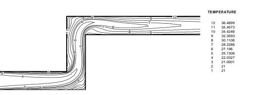
(b) H/W=3, U<sub>in</sub>=0.5m/s, To=40 °C
