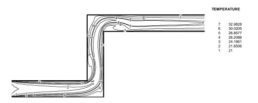
(c) H/W=4, Uin=0.14 m/s, Tw=35 °C
