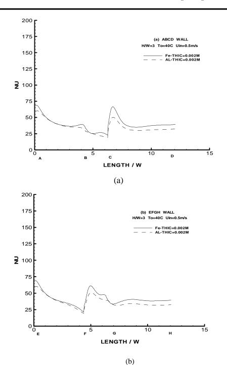
Figure 13 Local Nusselt number distribution along the upper and lower duct walls for turbulent flow, H/W=3, Uin=0.5m/s, To=40°C, Thick=0.002m, and (Fe-Metal and Al-Metal).
