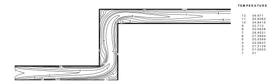
(c) H/W=4, U<sub>in</sub>=0. 5m/s, To=40 °C Figure 8 Contours of temperature distribution for turbulent flow, heat conducted at wall boundary, (a-H/W=2, b-H/W=3, and C-H/W=4), To=40 °C, and U<sub>in</sub>=0.5m/s.
