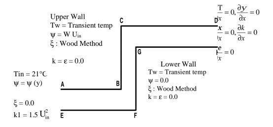
Figure (3) Boundary conditions for turbulent flow at H/W=3.
