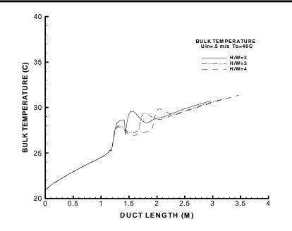
Figure 9 Variation in air bulk temperature along the Fe- duct for turbulent flow,  $U_{in}$ =0.5m/s, To= 40 C, and (H/W=2, 3, and 4).
