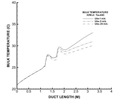
Figure 10 Variation in air bulk temperature along the Fe-duct for turbulent flow, H/W=3, To=40 $^{\circ}$ C, and (U<sub>in</sub>=1, 0.5, and 0.35m/s).
