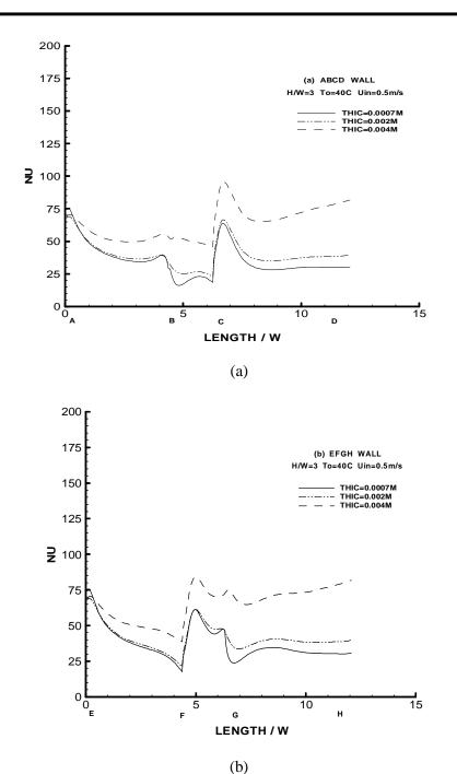
Figure 12 Local Nusselt number distribution along the upper and lower duct walls for turbulent flow, H/W=3, To=40°C,  $U_{in}$ =0.5m/s, and (Thick=0.0007m, 0.002m, and 0.004m).
