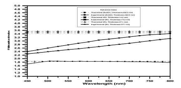
Figure (1) Experimental and theoretical refractive index versus wavelengths for Scandium Oxide and Rhodium.
